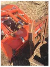
Tschetter adapted a 3-pt. pallet fork to fit the 4-ft. bucket on his 23 hp. Kubota loader tractor.
