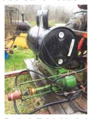
Hempel used a 55-gal. plastic barrel and the grain conveyor off an old combine to build this 3-pt. mounted cube feeder.
