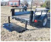
Cerveny built a 4 by 8-ft. trailer and added an old Tommy Gate lift and 12-volt deepcycle battery to make trailer easy to load.
