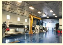
Jeff Hoeft converted his farm shop to build customized countertops out of stone slabs, using an Italian-made computerized CNC saw to cut the stone.
