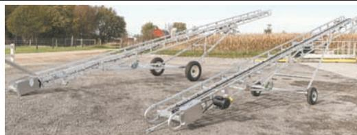
Dalam bale elevators have lightweight aluminum frames and are ideal for handling small square bales.
