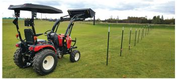
Tee-Post driver hangs from loader bucket. Post slips into driver barrel, which swings freely on swivel, allowing gravity to align posts. By inserting a pin to lock onto fencepost notch, posts can be pulled quickly with driver.
