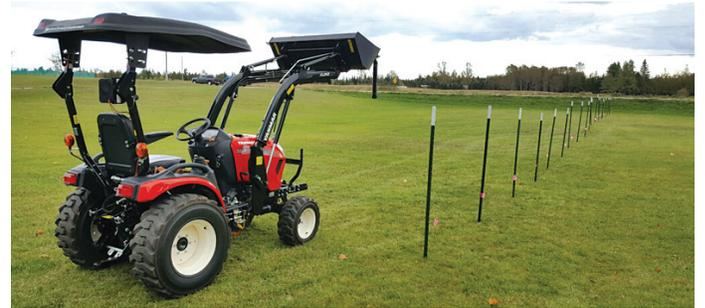
Tee-Post driver hangs from loader bucket. Post slips into driver barrel, which swings freely on swivel, allowing gravity to align posts. By inserting a pin to lock onto fencepost notch, posts can be pulled quickly with driver.
