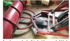
Loader can also be fitted with an angled blade that Stemmann welded to a semi-circular frame. It pins onto another frame that bolts onto loader arms.
