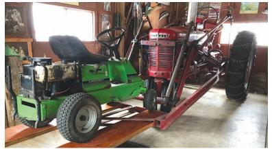
Two 5-ft. long boards, attached between loader arms, make it easy for Stemmann to work on riding mowers.
