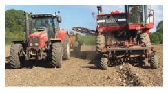
conveyor that carries them back to a rotating screen that cleans the rock and feeds it to an elevator that unloads to a following wagon.
