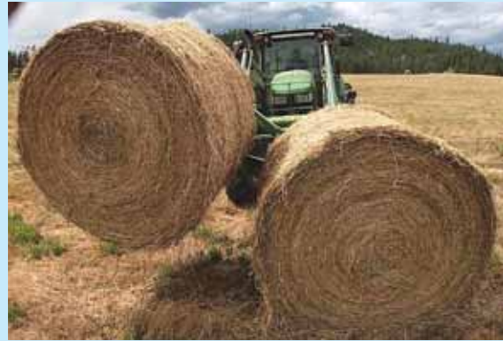
After spearing a bale, it can be swung out of the way to spear a second bale, saving handling time.
