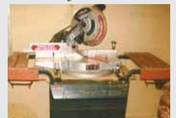
**Frank Brossart, Rugby, N. Dak.:** “I converted an old gas grill that didn’t work any more into a portable table saw stand. I replaced the grill with a piece of 1/2-in. thick plywood and set the saw on top of it.
