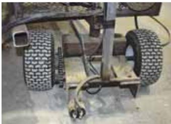
Electric drive support base with pivot point and drive wheels.
