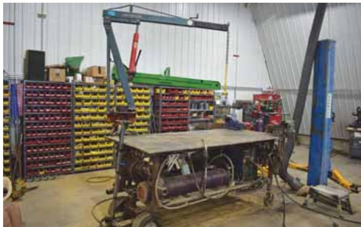
Mobile welding table with hoist, vises and under frame storage.
