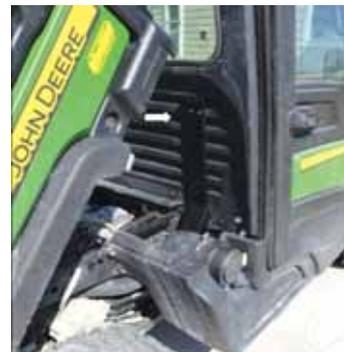
Ken Hall made a new duct that connects to the air intake tube on the engine and extends up about 18 in. between the cab and the box.
