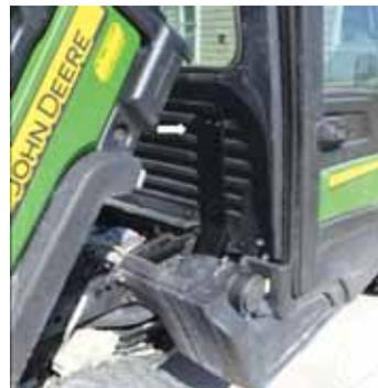
Ken Hall made a new duct that connects to the air intake tube on the engine and extends up about 18 in. between the cab and the box.
