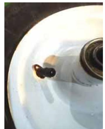
"I just install a hog ring on the valve stem, preventing it from ever being sucked into the wheel," Bunniss explains.
