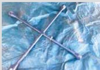
**John Rochester, Deerfield Beach, Fla.:** "When using a four-way wheel wrench, it saves a lot of aggravation to mark the size used most often."
