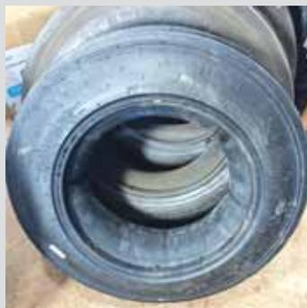
**John Humeniuk, Baudette, Minn.:** "Keep spare tires in shape with pumped up inner tubes. If new tires have flattened out in storage, the inner tube gets them back in shape, making them easier to mount on rims."
