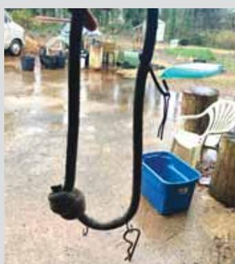
"This is a loop of 1/2-in. rope. It's fitted with three different sizes of S hooks. It works much better than pliers for pulling cotter pins and clips."
