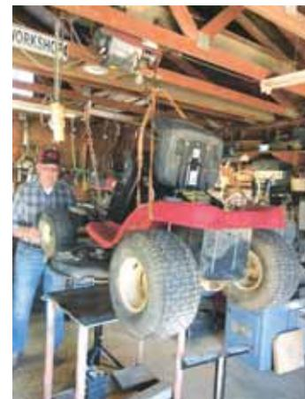
**With the riding mower in place beneath the winch, Wells attaches the spreader bar, lowers the winch cable and hooks it to the spreader bar. After raising the cable just enough to tension the chains, he loops the ratchet strap under the rear fenders of the riding mower.**
