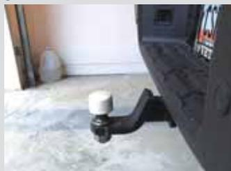
**Jeff Binion, Newnan, GA:** "I put a 2-in. pvc pipe cap on my truck's trailer ball. The rear camera picks up the cap much better when backing up. Just ream it out a little
