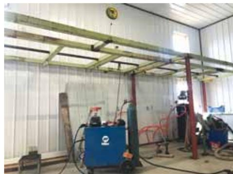
**Scott Ravenkamp built a shop loft using an old weeder frame with pallet racking used for legs.**
