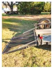
Smith used standard springs and hardware to ease the load of his trailer tailgate.
