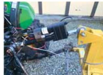
Top link on 3-pt. replaced with 12-volt actuator.
