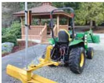
Laine used the output from a laser receiver to make his own leveling system.
