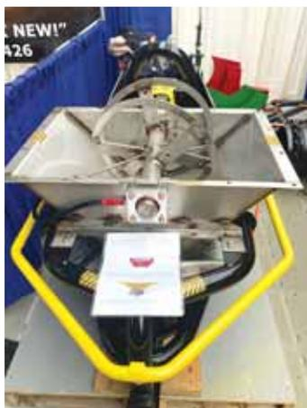
Spreader is shown without the hopper, revealing the pto driven auger inside.
