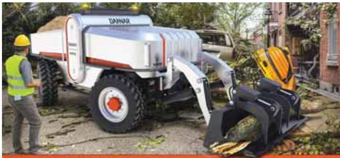
MPS unit can be run from the operator's cab using a joystick, from the ground with remote control, or programmed to move autonomously by accessing GPS coordinates.
