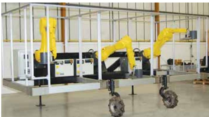
Each robot can harvest up to 1,200 heads per hour versus 515 per laborer. Each head is cut at a specified size and height versus assessment by eye and experience with manual harvest.
