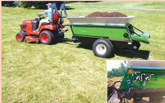
MultiSpread 320 with light material sides spreading compost. Inset shows hydraulic drive for conveyor and apron.
