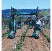
Gantry design works like a framework mounted on two motorcycles with independent steering. Mirror image sides are connected at their tops by tubes that slide into and rotate inside a center tube.
