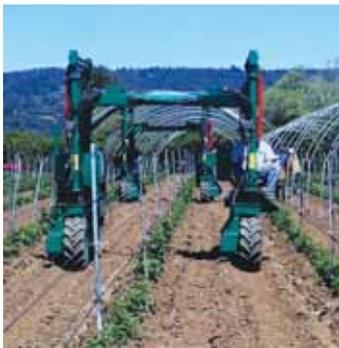
**Gantry design works like a framework mounted on two motorcycles with independent steering. Mirror image sides are connected at their tops by tubes that slide into and rotate inside a center tube.**
