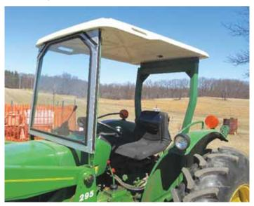
Fisher made a front frame to support the roof and provide a windshield opening out of 1-in. angle iron. It's bolted securely to the upright brackets on the tractor's 295 loader frame. The rear of the roof is mounted to the tractor's roll bar.
