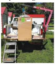
A 2 1/2-ton scissor jack under the bumper supports it if the payload weighs 300 lbs. or more. Patterson says the hoist doesn't obstruct the width of the bed so he can still load plywood sheets or other wide items.
