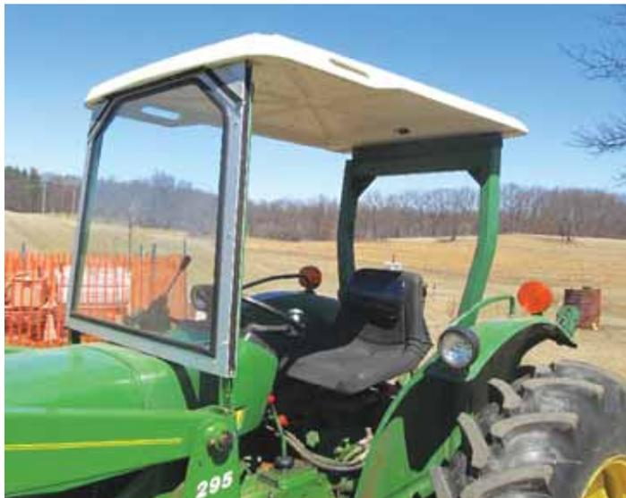
**Fisher made a front frame to support the roof and provide a windshield opening out of 1-in. angle iron. It's bolted securely to the upright brackets on the tractor's 295 loader frame. The rear of the roof is mounted to the tractor's roll bar.**
