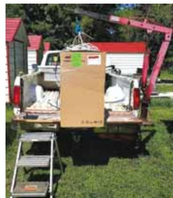
**A 2 1/2-ton scissor jack under the bumper supports it if the payload weighs 300 lbs. or more. Patterson says the hoist doesn't obstruct the width of the bed so he can still load plywood sheets or other wide items.**
