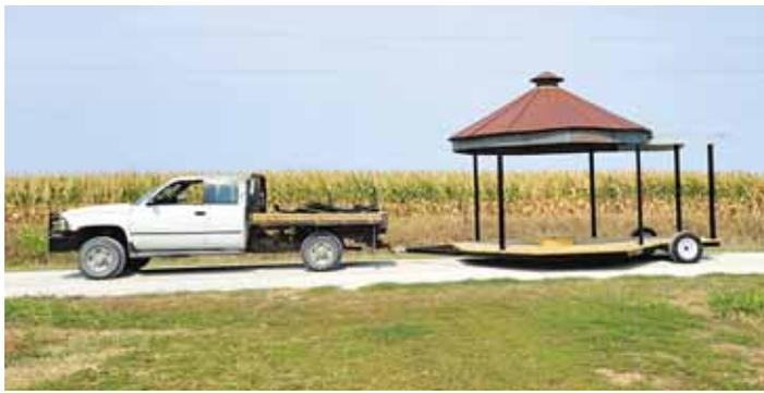
Clark built a 13-ft. 8-in. octagon-shaped base frame using 2 by 4-in. rectangular steel tubing. The frame rides on a 3,500-lb. axle and two 15-in. wheels. He used additional frame material to build a tongue, hitch and vertical posts to support the roof.
