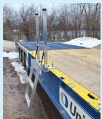
Trailer ladders made of aluminum fit into existing stake pockets and stay free of trailer sides.
