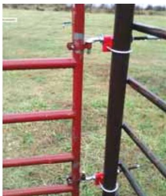
**EZ Hinge brackets are made from heavy-duty, 1/2-in. steel plate and schedule 40 steel pipe. Mounting gates requires only a tape measure, a 9/16-in. socket wrench and a crescent wrench.**
