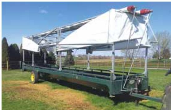
**A canopy system built on a portable feed trough is used to shelter horses during weddings, auctions and other events.**
