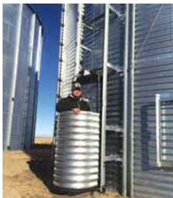
**When used with the Skytrack system, the Skylift elevator can be used on multiple bins.**
