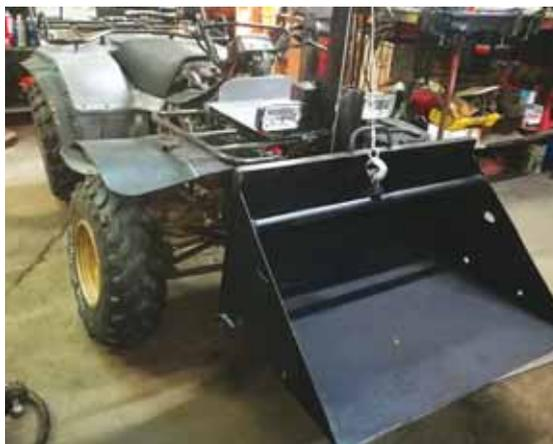
Heron figures the bucket can easily handle up to 200 lbs. He made it by cutting an old 3-ft. truck toolbox on the diagonal and adding a pipe to attach the winch cable.
