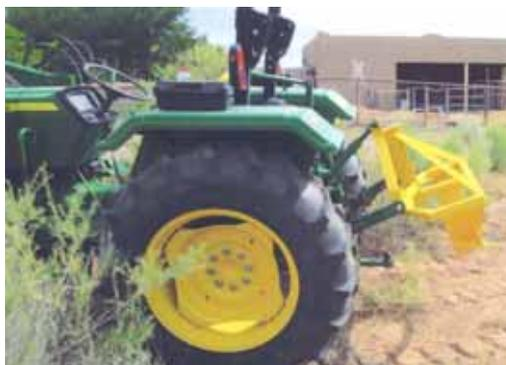
"Brushband" uses a curved blade connected to a 3-pt. hitch that removes brush with minimal soil disturbance.
