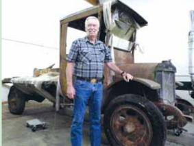
LaPlant carefully documents everything by taking photos and marking parts. Removing the rotting wooden frame of the cab on his new project, a 1926 truck, requires extra care so a pattern for a new wood frame can be made.
