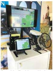
Control is offered by a tablet-based interface. The user can set a field plan, establish staging locations, adjust speeds, monitor location activity and command the tractor pulling a grain cart to sync with the harvester.
