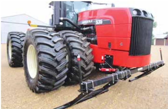
Front-mount Stalk Smasher has a 5-in. square toolbar and uses a hydraulic cylinder with 14-in. lift for ground clearance for the smasher bars that protect tires from field debris.
