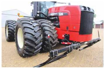
Front-mount Stalk Smasher has a 5-in. square toolbar and uses a hydraulic cylinder with 14-in. lift for ground clearance for the smasher bars that protect tires from field debris.
