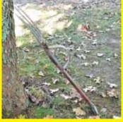
Being almost 80 years old and with a back that doesn't work as well as it used to, I couldn't stand to bend over a digging fork anymore. I replaced the wooden handle on the fork with a metal one and attached a broken tooth from a spring tooth harrow on the bottom side to act as a fulcrum. Now I can get down on my knees and dig potatoes. Sure saves the old back. (Mike Frantz, Seymour, Mo.)
