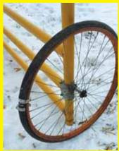
I welded a bolt to a bicycle wheel and attached it to the end of a gate, so it rolls back and forth. I stretched a piece of 3/4-in. hose around the wheel rim, held in place with hose clamps. You could also just use a wheel with the tire still in place. The big wheel works well on uneven ground. (Fritz Groszkruger, Dumont, lowa)
