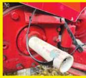
I recently bought an old tractor that did not have a pto guard. I made a pto shield using heavy-duty pvc and a reusable wire tie. I have read that if you get caught in a pto at 540 rpm your brain doesn't know you are in trouble until you have made four full revolutions. Some of us old guys may take even longer. (Gary Swensen, Yankton, S. Dak.)
