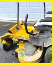
I installed a post on my zero-turn lawnmower to make it safer to mount and dismount. It cost \$25 total for a 24-in long piece of threaded 3/4-in. black pipe, a floor flange, four 5/16-in. hex head bolts and nuts, an end cap, close nipple, and an elbow bend. I tack welded each end of the close nipple to ensure rigidity. (Jack Norris, Lafayette, Ind.)
