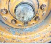
**Carl Stoloski, Appleton N.Y.:** "I put a used oil filter on my tractor front hub as a dust cap."
