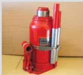
LeRoy Momper, Fredonia, Wis.: "Whenever I wanted to use my bottle jack I would have to search for the handles. I solved the problem by clamping two pieces of conduit to the jack. Now the handles are always with the jack and the conduit does not interfere with operating the jack."
