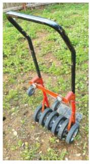
Adding additional wheels with PVC spacers makes a hand truck easier to use on soft ground.
