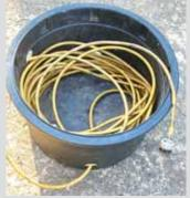
John Rochester, Deerfield Beach, Fla.: "I use plastic flowerpots to hold extension cords. I drill two holes, one near the bottom and the second on the opposite side and higher up. I put the extension cord inside and pull a few feet out of the bottom hole and coil the rest inside. You can just pull out what you need and they're stackable for storage."
