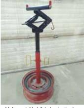
McLaen drilled 2 holes in the lower pipe and welded nuts to the whole surface. D-handle set screws fabricated from scrap bolts lock the inner pipe in place after it's adjusted.
