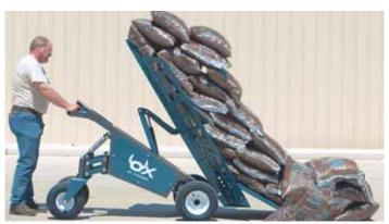
The 1,000-watt, 36-volt power supply provides a run time of 8 hrs. continuous use and up to 3 mph speeds.
