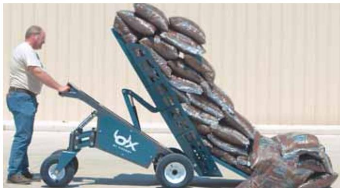
The 1,000-watt, 36-volt power supply provides a run time of 8 hrs. continuous use and up to 3 mph speeds.
