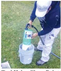
In less than a minute and about 3 gallons of water, the roller cover is clean and dry enough for immediate reuse.
