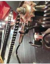
Stroke count sensor on knotter chain handle.
