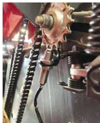
Stroke count sensor on knotted chain handle.
