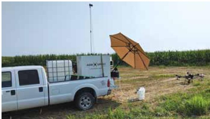
Agri Spray Drones builds a self-contained metal Launch Box on a pallet type frame that carries a spray drone and its control system along with mixing tanks and a refilling pump.
