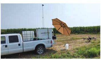
Agri Spray Drones builds a self-contained metal Launch Box on a pallet type frame that carries a spray drone and its control system along with mixing tanks and a refilling pump.
