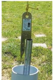
When lowered down through a pipe via a retrieval line, one of The Fetch jaws slides into the opening of the broken pipe and grabs it there, while the other grips it on the outside.
