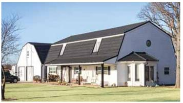
Metal roof panels of 26-ga. stone coated steel measuring 3 ft. by 20 in. feature an acrylic base coat and have the same stone granules used in asphalt shingles.
