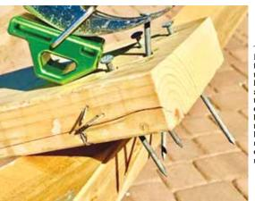
The Rizer Hammer fits over a traditional hammer claw and elevates the point of contact between the nail and hammer, making it easier to pull nails.
