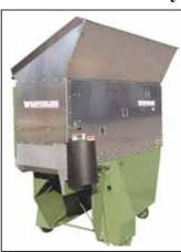
Mulch Bagger was designed to be an improvement from two workers with a shovel and a bag. One person can fill up to 200 bags per hour.
