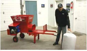
The double screw system can be adjusted to increase or decrease compaction of silage entering the 26 1/2-in. dia., 44-in. long bags.
