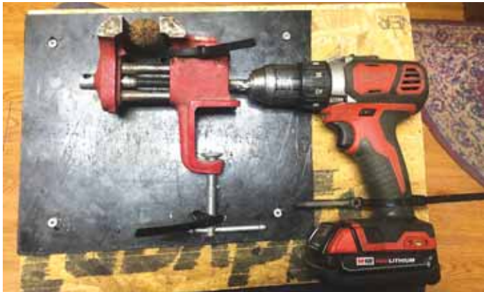
Hawkes combined a battery-powered drill with a small clamp-on vise to make a nutcracker.
