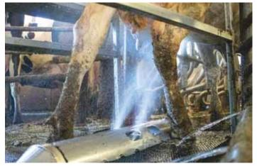
TurboSpray is a walkover, floor-mounted, air-assisted, teat preparation system mounted near a parlor's entry or exit lanes.
