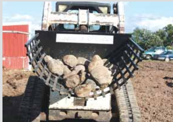
U-shape bucket design doesn’t allow rocks to get stuck.
