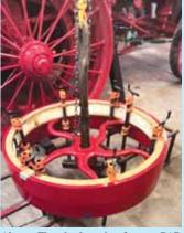
Above: Fly wheel casting from a CAD drawing. Below: Before restoration.
