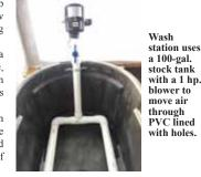
a 100-gal. stock tank with a 1 hp. blower to move air through PVC lined with holes.
