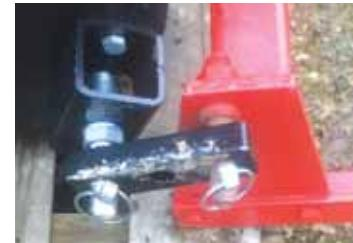
**Yax uses dog bone connectors between the pins on the bucket and the attachments and a steel bar pinned to the clevis in place of an adjustable top link.**
