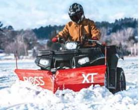
Boss V-Plow XT uses a skid-plate mount and can adjust up to 30 degrees.
